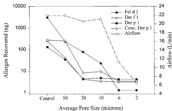
**FIG 3.** Allergen recovered from filter after testing fine woven fabrics with 1.0 g of dust containing 510 µg/g Fel d 1, 5.5 µg/g Der f 1, 3.7 µg/g Der p, 1 or 26.9 µg/g concentrated Der p 1. The amounts of allergen recovered from the 6-µm and 2-µm fabrics reflect the lower limit of the assay. The control was a used cotton sheet (laboratory control).
