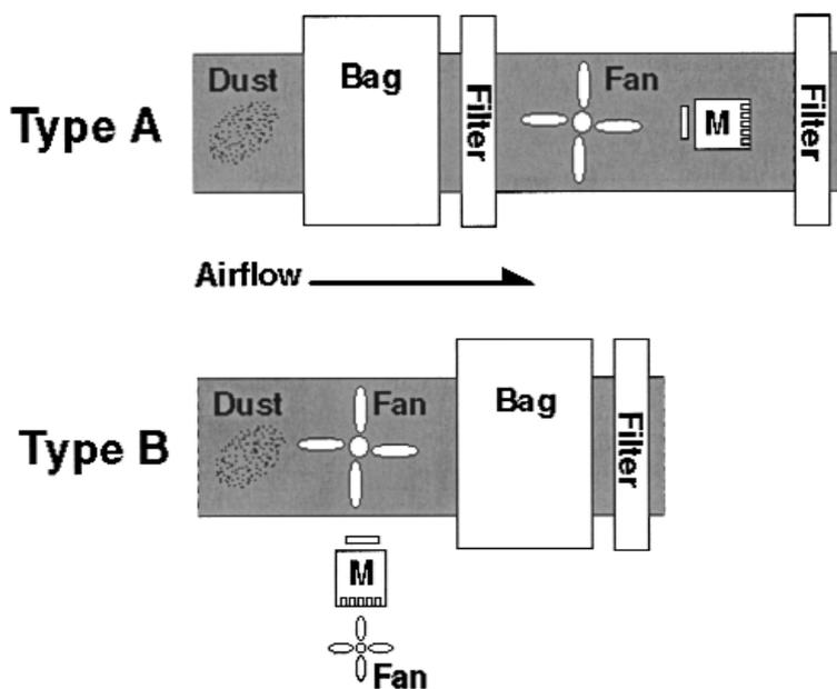
**FIG 4.** Two predominant designs used by vacuum cleaner manufacturers. Both designs allow airborne particles to pass through the bag and a filter leading out of the machine. In design *A* airflow passes around the motor before exiting through the exhaust filter. In design *B* the motor is located outside the flow of air through the machine, and particles emitted from the motor are driven into the environment by the fan used to cool the motor. *M*, Motor.
