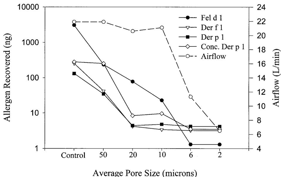
**FIG 2.** Allergen recovered from filter after testing fine-woven fabrics with 1.0 g of dust containing 510  $\mu\text{g/g}$  Fel d 1, 5.5  $\mu\text{g/g}$  Der f 1, 3.7  $\mu\text{g/g}$  Der p 1, or 26.9  $\mu\text{g/g}$  concentrated Der p 1. The amount of allergen recovered from the 6  $\mu\text{m}$  and 2  $\mu\text{m}$  fabrics reflects the lower limit of the assay. The control was a used cotton sheet (laboratory control).
