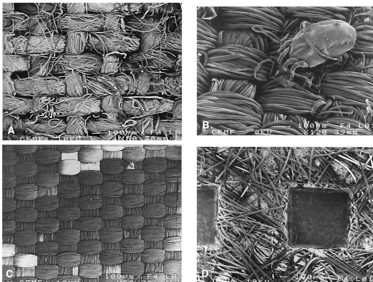
**FIG 5.** Scanning electron microscope pictures of four fabrics: (A) cotton sheet with large pores (laboratory control), (B) dust mite on fine woven fabric (Pristine, 6  $\mu$ m fabric), (C) very tightly woven (2  $\mu$ m) fabric used for surgical gowns, and (D) nonwoven material showing heat welding (Softtek, Medibed) (see Table I for details).
